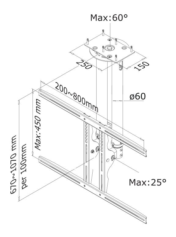
Neomounts Measuring unit: mm
